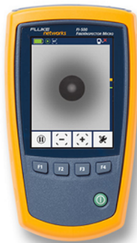
FI-500 displaying a clean fiber endface
