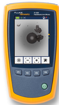
FI-500 displaying a dirty fiber endface
