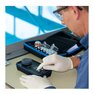
Multi-parameter photometer with Bluetooth interface / PC software / Cloud service / Cross-system synchronization of measured values / Up to 7 selectable parameters / For measuring e.g. pH, alkalinity, chlorine, cyanuric acid / Storage of measured values
