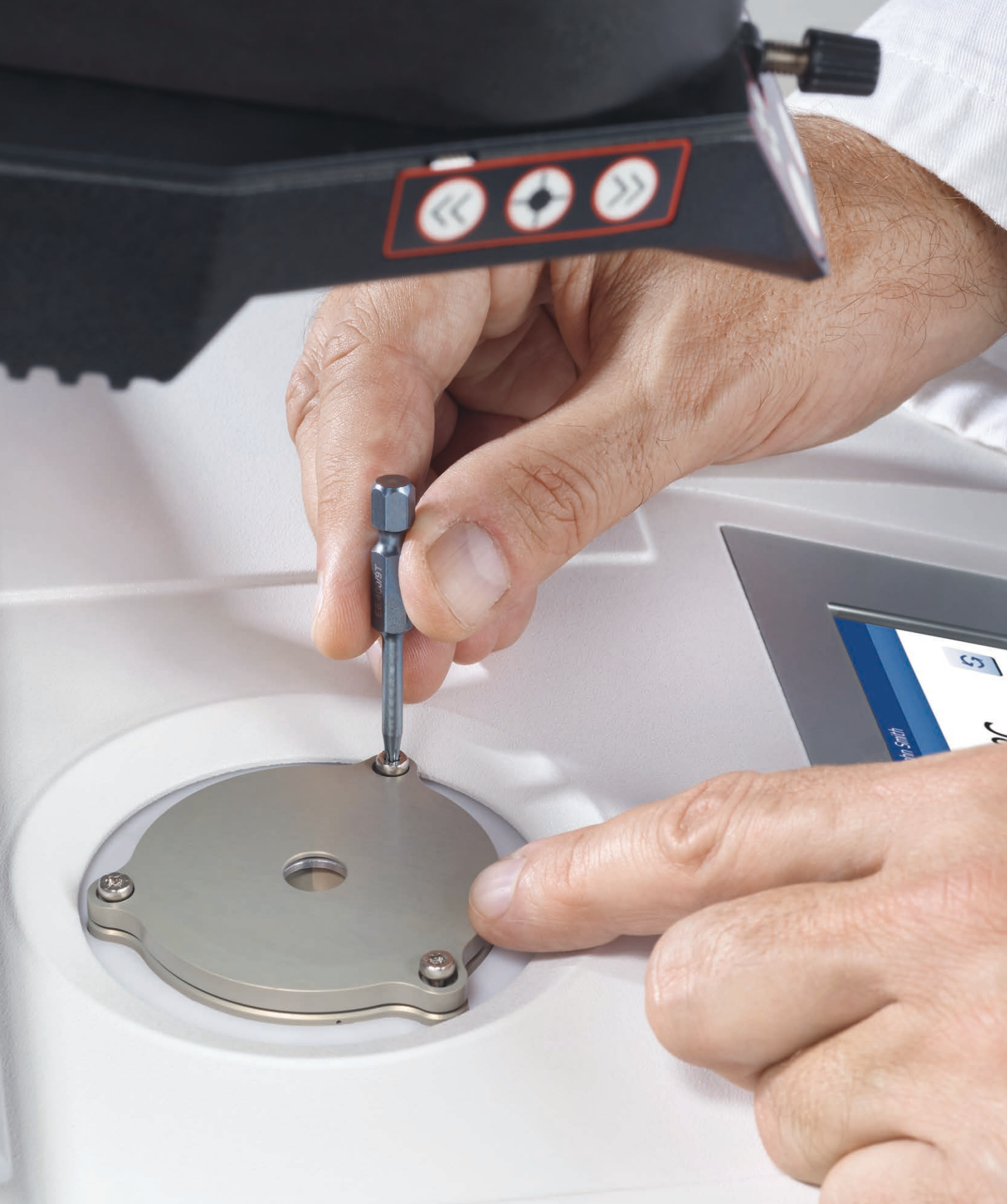
The screw closure lid ensures oxygen-free conditions. It tightens the measuring cell and prevents any gas exchange with the surroundings.
