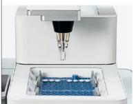
For sensitive samples, a lid can be placed on the crucible and automatically removed before the measurement or, for hermetically sealed crucibles, pierced just before the measurement starts.
