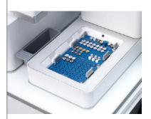
The environmentally-controlled crucible chamber stores up to 96 sample crucibles and 7 reference crucibles for continuous measurement.
