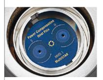
The single furnace power compensation mode is enabled by two heaters integrated into the sensor. During a measurement, the  $\Delta T$  between the sample and reference positions is compensated by the heaters, so  $\Delta T=0$ .
