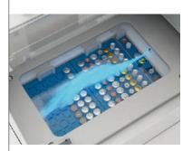
When using the sample robot, a large number of samples can be stored in the crucible chamber.
