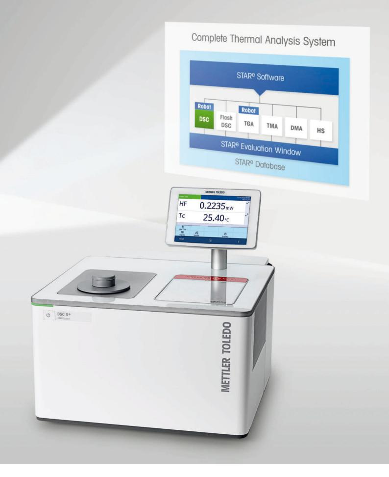
A complete thermal analysis system consists of six complementary measuring techniques, each bringing fast and accurate results. Additional knowledge and information about your sample can be obtained by using a variety of hyphenated techniques.
