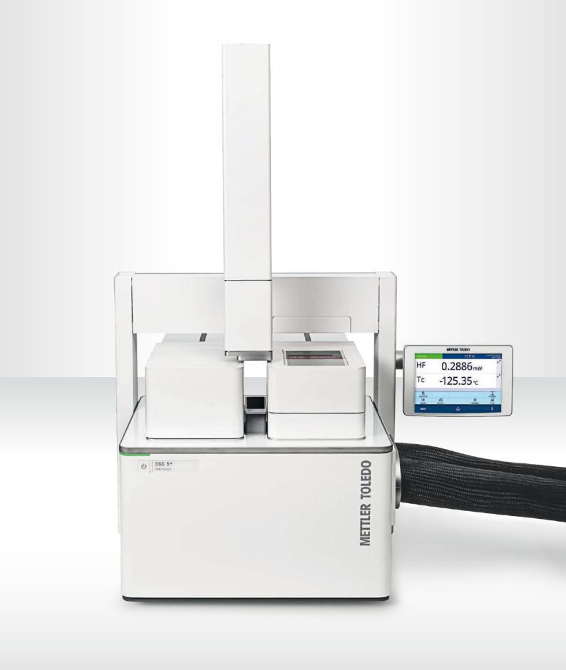
A more productive DSC — High-capacity sample robot with 96 sample positions, exchangeable reference, crucible lid piercing and environmental control is combined with FlexCal<sup>TM</sup> and the powerful S**TA**R $^{\rm e}$  software, including AlWizard<sup>TM</sup>, to increase your laboratory's efficiency.
