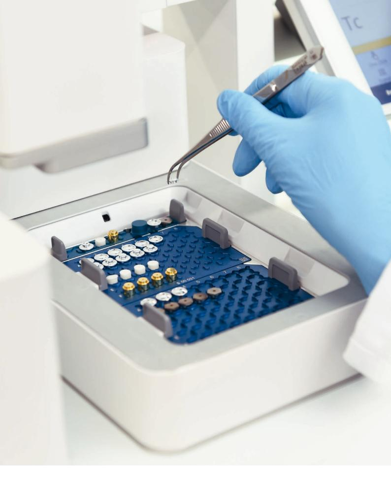
Removable sample and reference crucible trays allow for easy sample preparation. The DSC 5+ will automatically identify the tray and select the correct sample for measurement.
