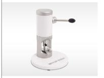
The press allows the pan to be sealed very easily. Under the pressure of the plunger the pan is cold welded, hermetically sealing with the lid. After changing plunger and die you can use the press for other crucibles.
