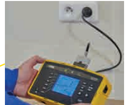
3-pole cable for direct measurements on 2P+E sockets.
