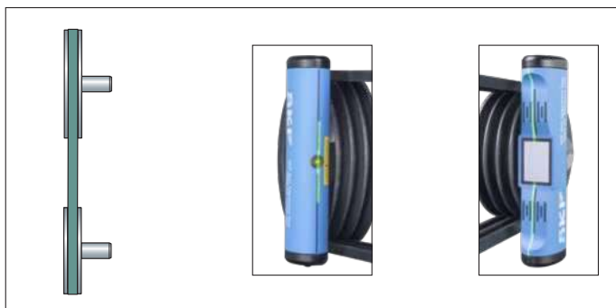
Figure 9 Pulleys perfectly aligned
