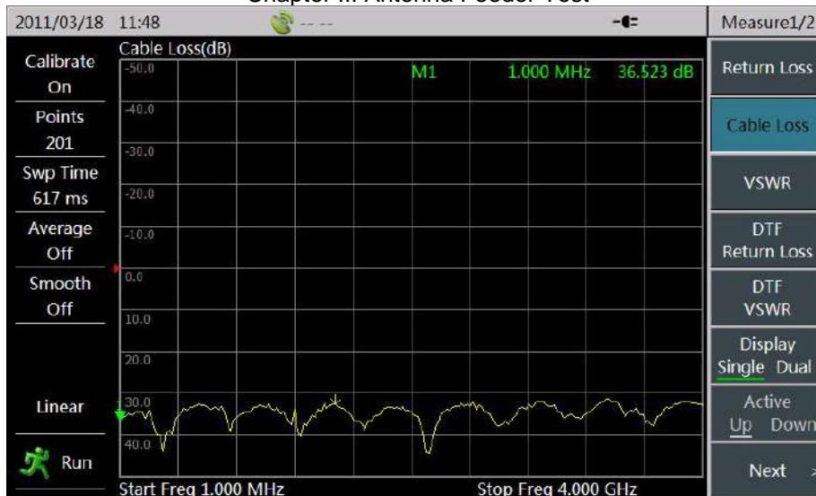
Figure 3-14 Cable Loss Measurement
