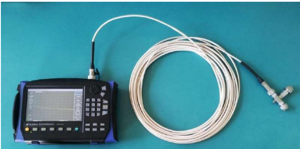
Figure 2-7 Connection Types for Cable Loss Test
