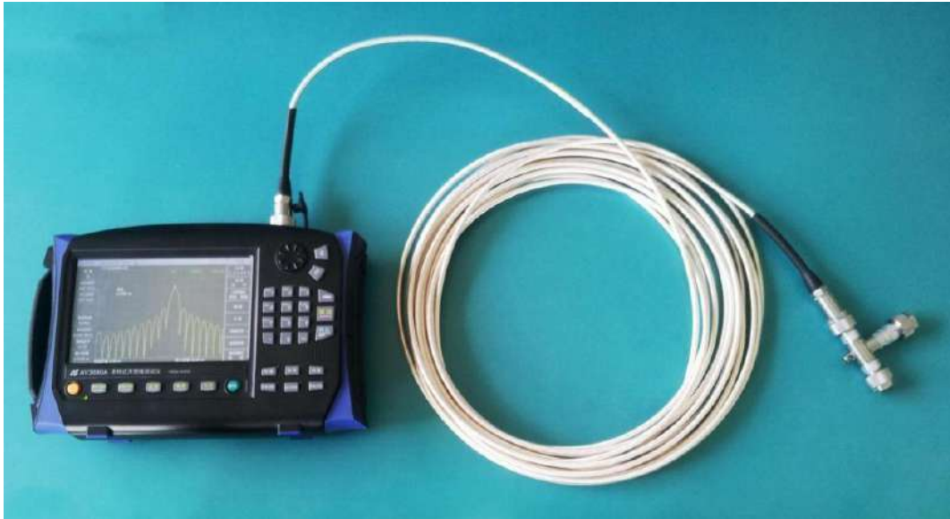
Figure 3-12 Connection for DTF Return Loss Test
