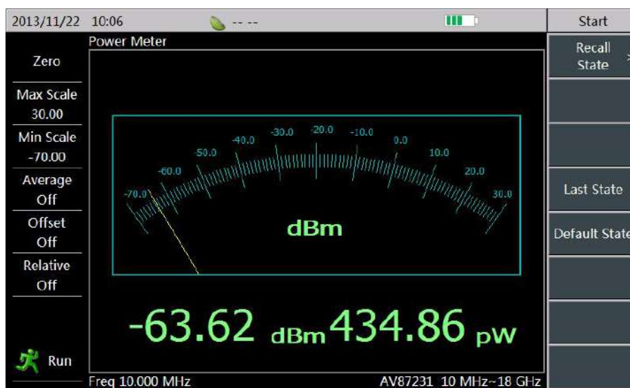
Figure 4-1 Power Test Interface
