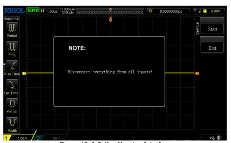
Figure 13-2 Self-calibration Interface
