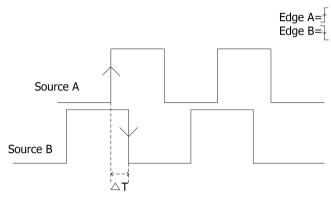
Figure 5-10 Delay Trigger
