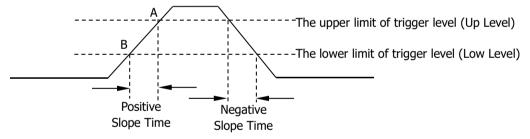
Figure 5-4 Positive Slope Time/Negative Slope Time
