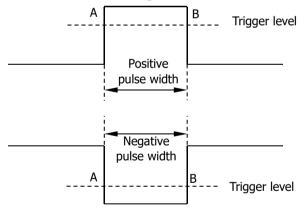
Figure 5-3 Positive Pulse Width/Negative Pulse Width
