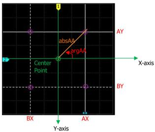
Figure 6-8 XY Cursor Measurement Definition
