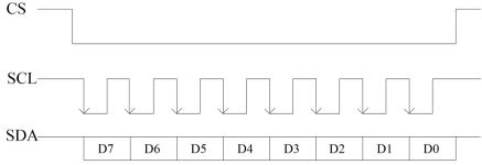
Figure 5-15 Sequential Chart of SPI Bus
