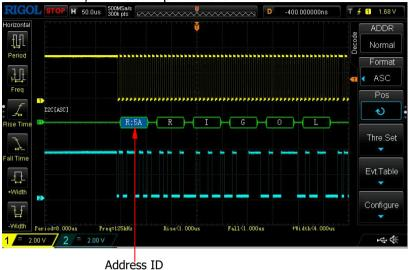
Figure 7-6 I2C Address Information during Decoding
