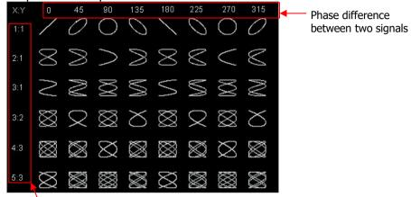
Frequency ratio between two signals
