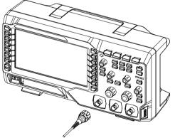
Figure 1-5 To Connect the Passive Probe
