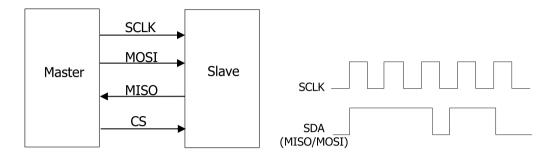
Figure 7-1 SPI Serial Bus
