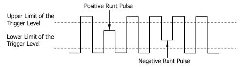
Figure 5-9 Runt Trigger
