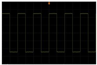
Figure 4-2 The Waveform after 256 Averages
