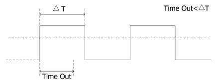
Figure 5-8 TimeOut Trigger
