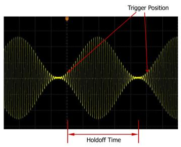
Figure 5-2 Schematic Diagram of Trigger Holdoff
