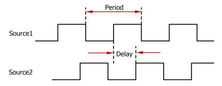
Figure 6-4 Delay and Phase
