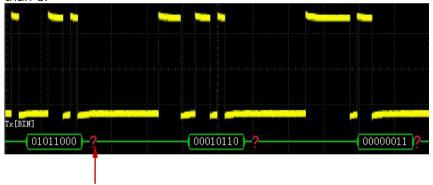
The stop bit is less than 1
