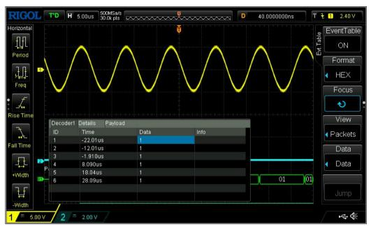
Figure 7-2 Parallel Decoding Event Table
