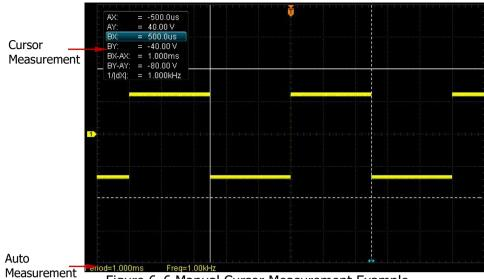
Figure 6-6 Manual Cursor Measurement Example
