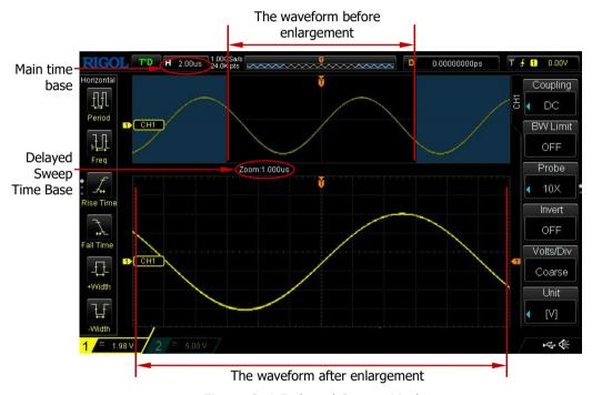
Figure 3-1 Delayed Sweep Mode
