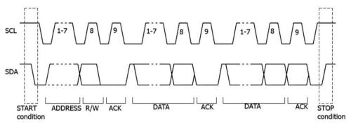
Figure 5-14 Schematic Diagram of I2C Protocol
