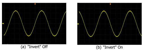
Figure 2-1 Waveform Invert
