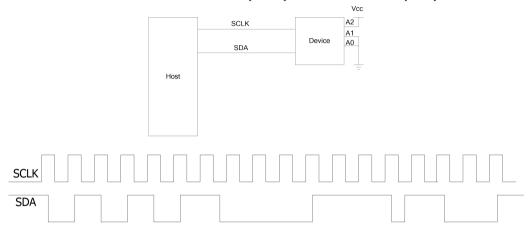
Figure 7-5 I2C Serial Bus
