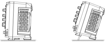
Figure 1-3 To Adjust the Supporting Legs
