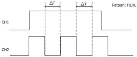
Figure 5-7 Duration Trigger
