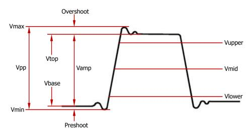
Figure 6-5 Voltage Parameters
