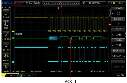
Figure 7-7 I2C Error Expressions during Decoding
