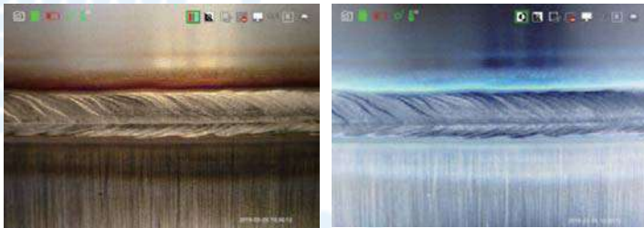
Normal Mode: HD image effect Negative Film Mode: Enhance the ability to compare and analyze the internal defects of the inspected objects.
