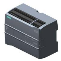
SIMATIC S7-1200, CPU 1215C, compact CPU, DC/DC/relay, 2 PROFINET ports, onboard I/O: 14 DI 24 V DC; 10 DO relay 2 A, 2 AI 0-10 V DC, 2 AO 0-20 mA DC, Power supply: DC 20.4-28.8 V DC, Program/data memory 125 KB
