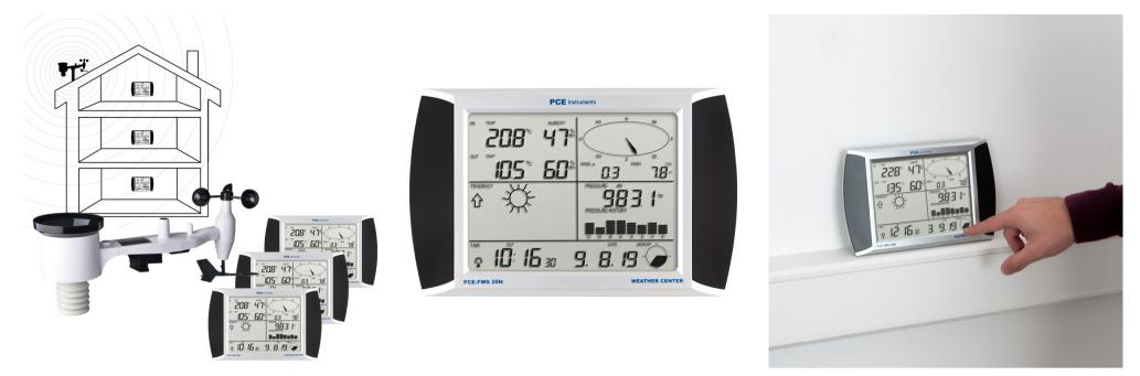
Radio weather station to determine the wind direction, wind speed, temperature, relative humidity and rainfall/ Adjustable alarm functions / USB interface / Analysis software / Solar module and batteries for powering the transmitter/ Transmission frequency: 868 MHz
