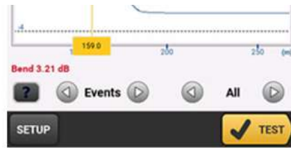
Bend as seen on an OTDR trace
