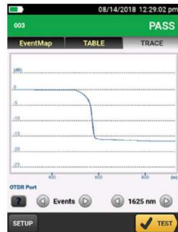
Splitter as seen on an OTDR trace
