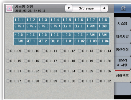
Figure 97) Status lamp indication
