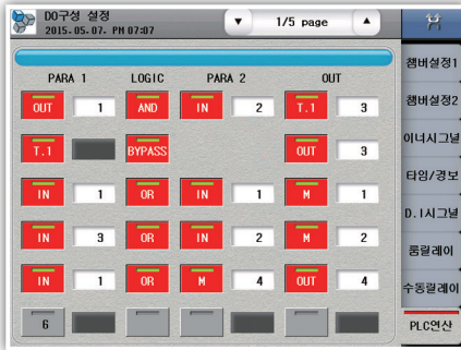
Figure 88) DO Configuration – PLC Operation
