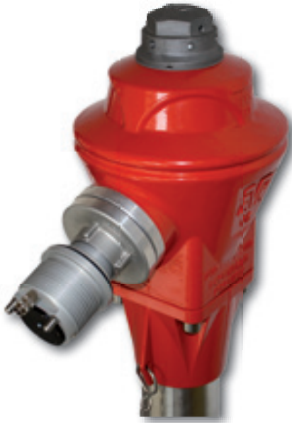
A Sebalog P-3, fastened on an above-ground hydrant
