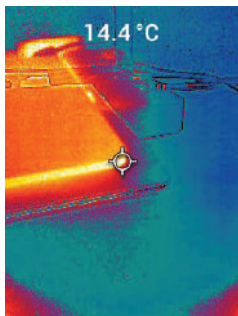
Figure 5.1 Combined Thermal and Visible Image (MSX®)
