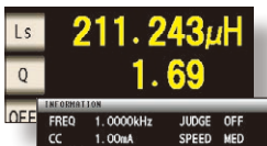
L and Q display screen (1 kHz, 1 mA constant current measurement)
